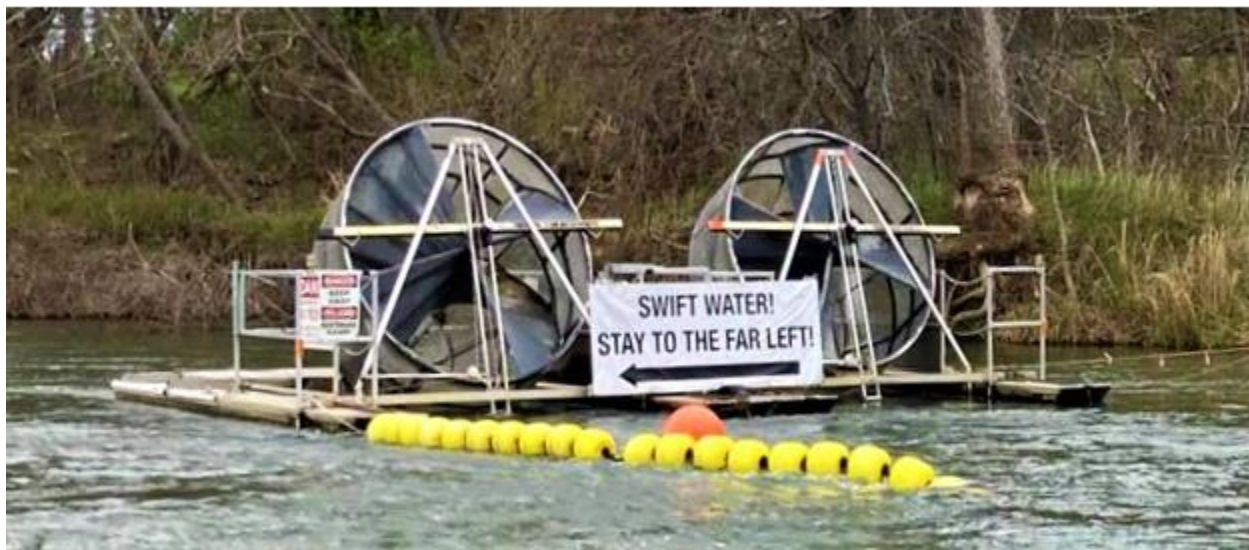
Figure 3: The two north channel 8-foot RSTs, Trap 8.1 (river right) and Trap 8.2 (river left), on the lower American River downstream of the Watt Avenue Bridge.
