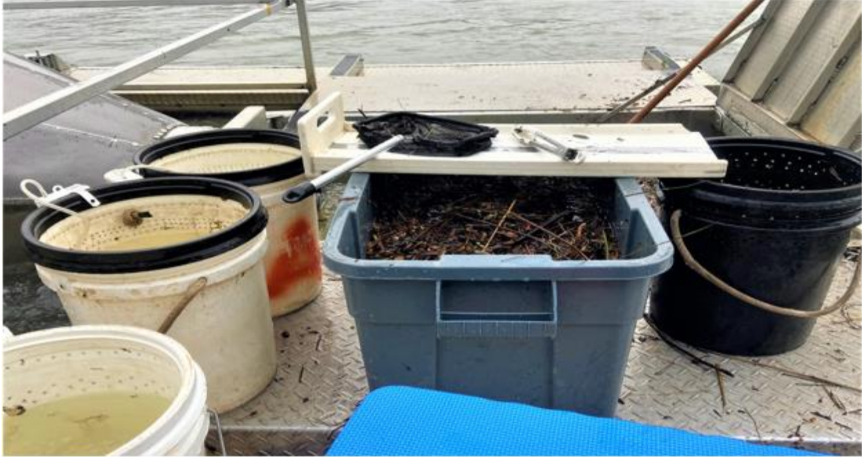
Figure 4: Trap workstation, consisting of an 18-gallon tub, multiple 5-gallon holding buckets, a measuring board, and tongs, on the lower American River.
